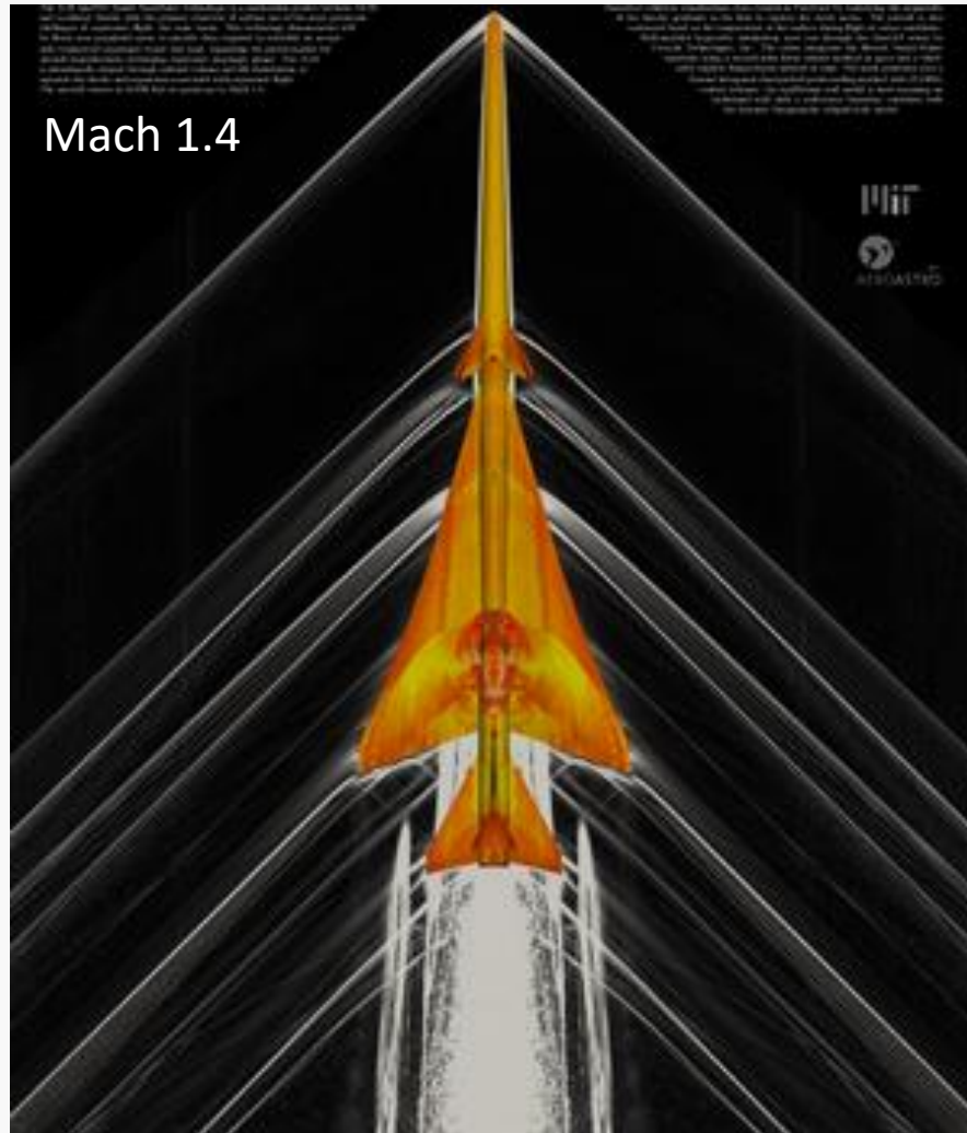
P0015: Numerical Schlieren of the X-59 QueSST (74th Annual Meeting of the APS Division of Fluid Dynamics 2021)
